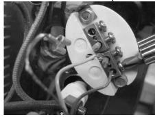
For 3 section kilns, you may also have to disconnect the 2 black wires between the middle section & Bottom section. You will need pliers and an allen key.
