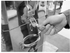
Move the kiln rings section by section.
