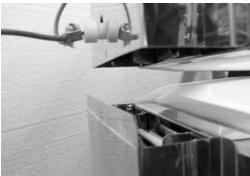
Remove the lid and put it aside. Then unlatch each of the clips around the body.
