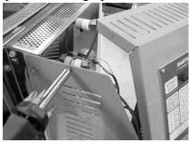
Use needle nosed pliers to pull the connectors off of the relays. Do not tug on the wires themselves.
